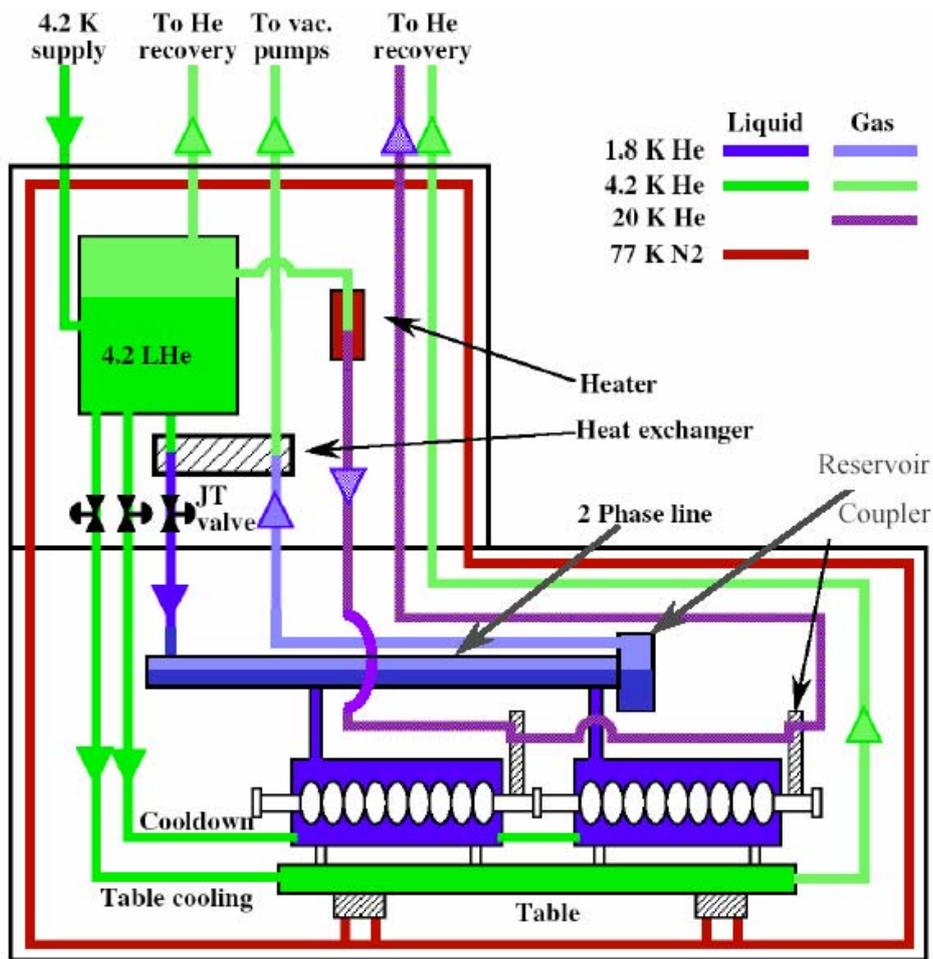
Figure 3: Layout of the HoBiCaT cryogenics. The vertical feedbox includes a liquid helium reservoir and 2 K cold box.
